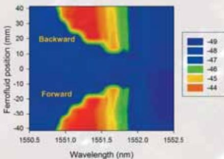
**Figure 1.** Spectral response of a chirped Bragg grating inscribed in a PCF that is infiltrated using ferrofluid
